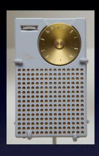
Regency TR-I transistor radio (1954) 4 transistors \$49.95, equivalent to \$427 today
